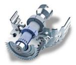
**Innovative Solutions to Complex Challenges:** "In this gear box cutaway two wheels mounted on one arbor are simultaneously grinding multiple bores and faces. "
